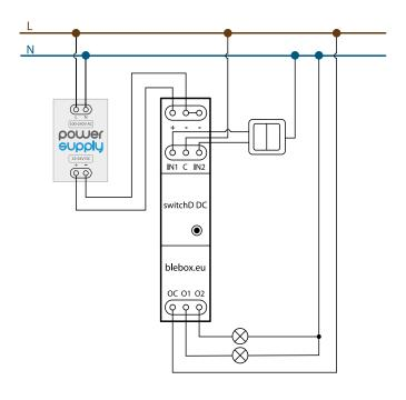
$\,$  6. Connection of other 230V AC peripherals (e.g. motion sensor, smoke sensor, water level sensor)
