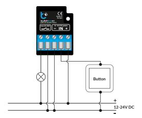
Separated controlled circuit, possibility to control 230V devices:
