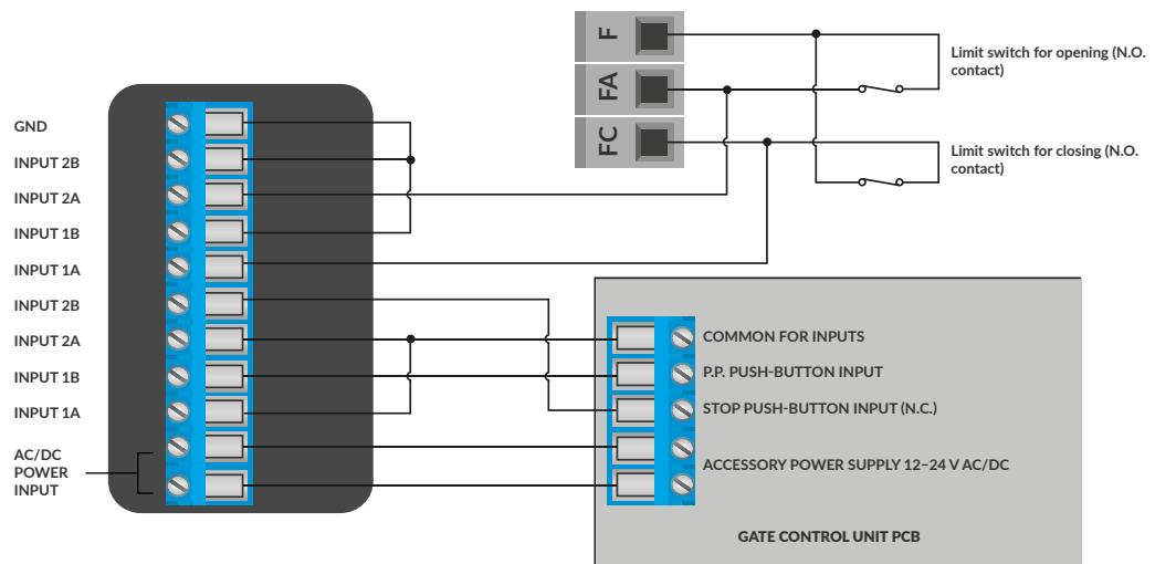
3. Wiring diagram for connection to a control unit with an output indicating the end position reached and an auxiliary output for closed-position signaling, based on the Somfy Control Box 3S RTS
