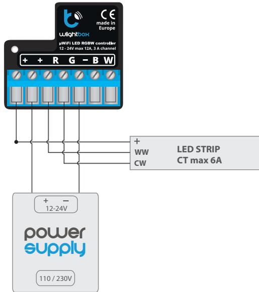
● wLightBox + 2 strips of 2-channel CT LED strip (CW/WW, CCT)
